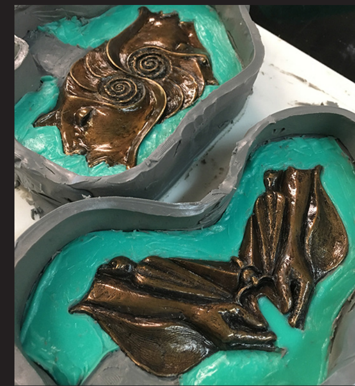
Bronze medals by Elaine Jaques in the process of mould making. These medals were sculpted in wax and cast directly. Moulds are being made to cast multiples.
