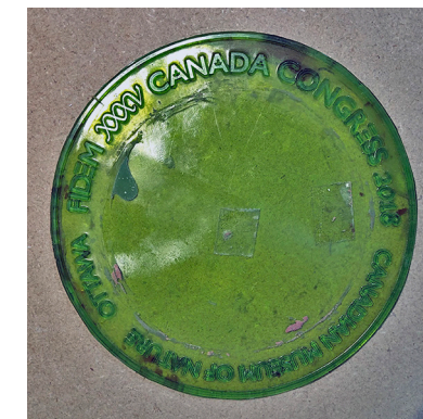
Rapid Prototyped Flexography plate. Work In Progress by Lorraine Wright.
