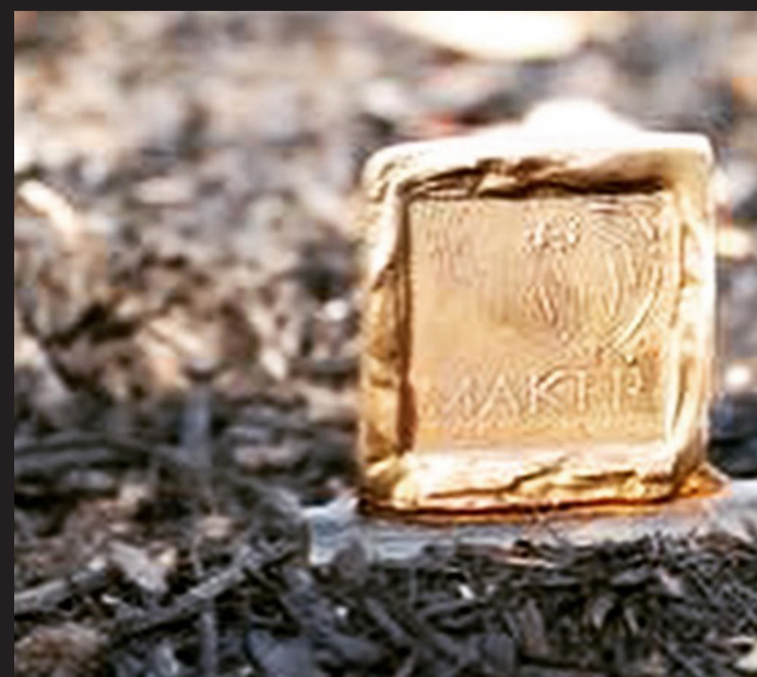
Example of bronze casting originally derived from a CNC milled rubber plate from a custom stamp manufacturer
